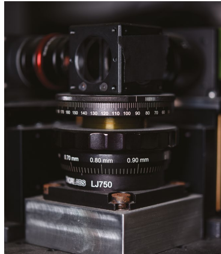
This camera system uses a beam splitter to capture the same scene with two different sensors. Because the same data can be collected using a high-resolution and low-resolution sensor at the same time, researchers can use this information to learn how to increase the resolution of the latter.
